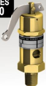
The Series 140 valve line is designed for air/gas safety. Compact in nature, yet rugged in all aspects of design and construction. The 140 series offers excellent fast acting reseating that minimizes loss of medium. High capacity flow rates.
